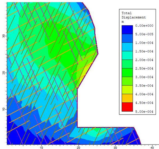
Fig. 9: The total displacement occurred in location 5 due to low curve cut slope.
