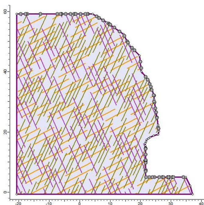
Fig. 3: Diagram showing geometry of the model and boundary condition used in the simulation (joint and other parameters are changed for different rock type and location).
