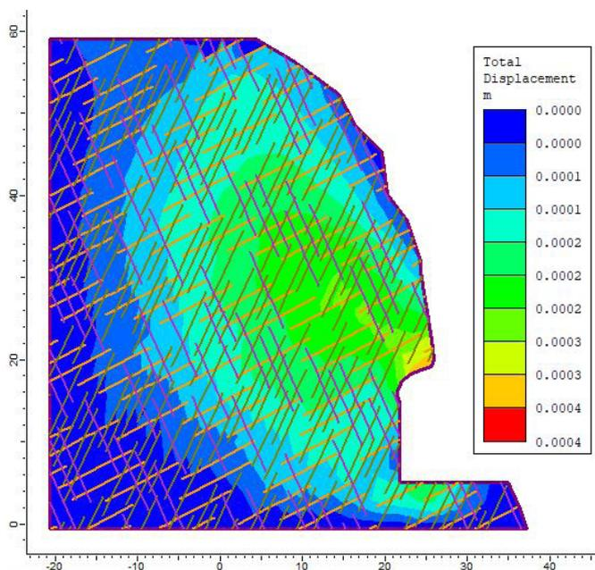
Fig. 5: Total displacement occurred in Location 1 due to high curve cut slope.
