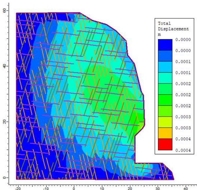
Fig. 7: The total displacement occurred in Location 2 due to straight cut slope.
